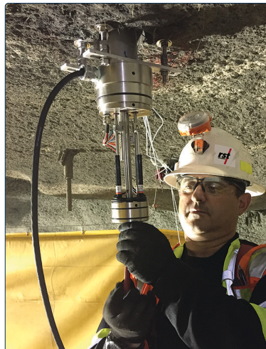
A Multi-Point Borehole Extensometer, with the Electrical Head cover removed, is being installed into the ceiling of an underground opening.
